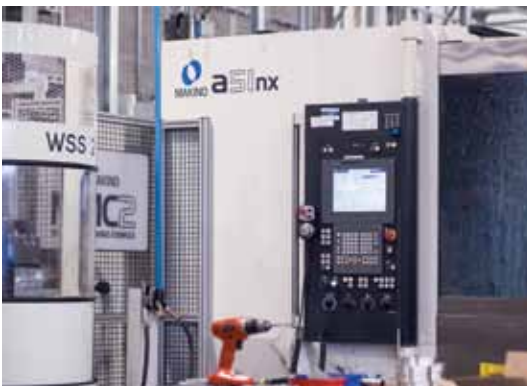
The Makino FMS with three a51nx horizontal machining centres and the MMC2 system with the MAS-A5 cell controller keep DDR competitive.
