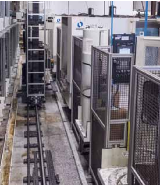
The Makino FMS with three a51nx horizontal machining centres and the MMC2 system with the MAS-A5 cell controller keep DDR competitive.
